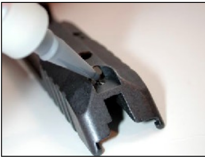
Figure 4. Initial application of adhesive.
