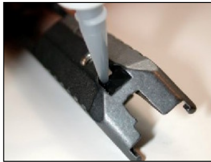
Figure 5. Spreading adhesive evenly.
